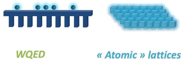
Figure 1: Left: atoms trapped on top of the comb waveguide [1]. Right: Quantum dots assembled in a 2D lattice.
